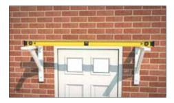
**1.5** Ensure second bracket is level and positioned correctly. Drill and secure as before.
