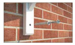
**1.4** Secure first bracket using the recommended fixings (Fischer SXR 10x100mm).
