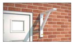
**1.2** To fit first bracket, mark positions for drill holes.
