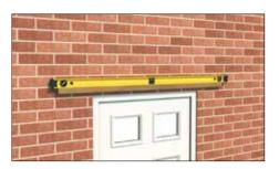
8.1 Fix a level batten at the desired canopy height.
