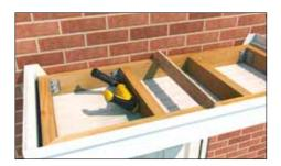
8.2 Rest soffit of canopy onto batten and drill all fixing holes. Drill bit size: M10
