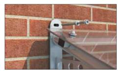
**4.4** Use a temporary fixing to hold canopy for levelling. Use the recommended fixing type (Fischer SXR 10x60mm).
