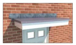
**8.10** Lead Flashing: If lead flashing is being used it must be pre-installed and folded down after the canopy is fully fitted and secured.
