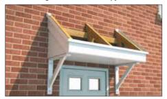
**6.2** Centre the canopy position, ensuring equal distance at either side, before pushing back to contact with the wall.
