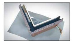
**2.1** Apply mastic sealant to the rear of the Flashing Upstand while on the ground. Use protective sheeting to front face of canopy.
