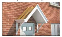
3.2 Centre the canopy position, ensuring equal distance at either side, before pushing back to contact with the wall.
