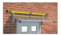
**4.5** Ensure canopy is level before marking the remaining fixing positions.
