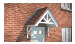
2.2 Centre the canopy position, ensuring equal distance at either side, before pushing back to contact with the wall.
