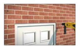
**4.6** Remove canopy before drilling the remaining holes. Drill bit size M10.
