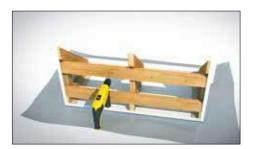
**6.1** Drill holes for fixing at min. 300mm centres, max. 450mm centres (drill bit size M10) First hole at min. 50mm from apex. Use protective sheeting to front face of canopy.
