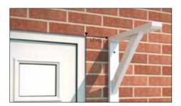
1.1 Determine canopy height: Level with door head, above door head etc. Width is determined by the canopy dimensions.
