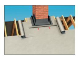
**6.2** Ensure main roof membrane is **LAPPED UNDER** the base membrane.
