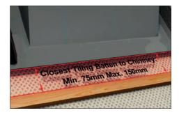
7.1 Before battens are secured 1No tiling batten must be fixed at front of chimney. This should be installed with a min 75mm to max 150mm below the GRP front edge flange.
