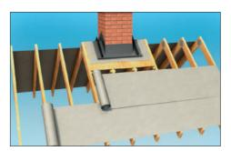
**6.1** Fit main roofing membrane around the dormer ensuring that it is **LAPPED UNDER** the base membrane.
