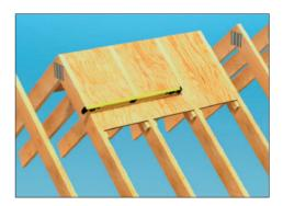
**1.4** Check to ensure the top of the fixing support boards and top of the rafters are level.
