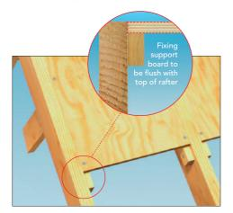
1.2 Ensure the position the battens is low enough to allow the fixing support boards to lay flush with top of the rafter when installed.
