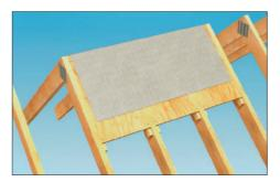
2.1 Install a base layer membrane over fixing support boards and secure as recommended.
