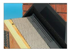
5.1 In order to secure the chimney to the support board drill 6mm holes spaced at 150mm centres along edge of GRP plinth as shown. Fix chimney to the support boards through pre-drilled holes using the recommended fixings.
