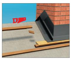
8.1 Where tiling battens meet GRP fixing flange, batten ends must be notched to ensure the batten sits flat and does not kick up.
